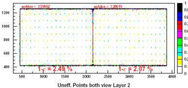
Inefficiency map of a Unit using reconstructed tracks for which neither phi nor eta were measured.
