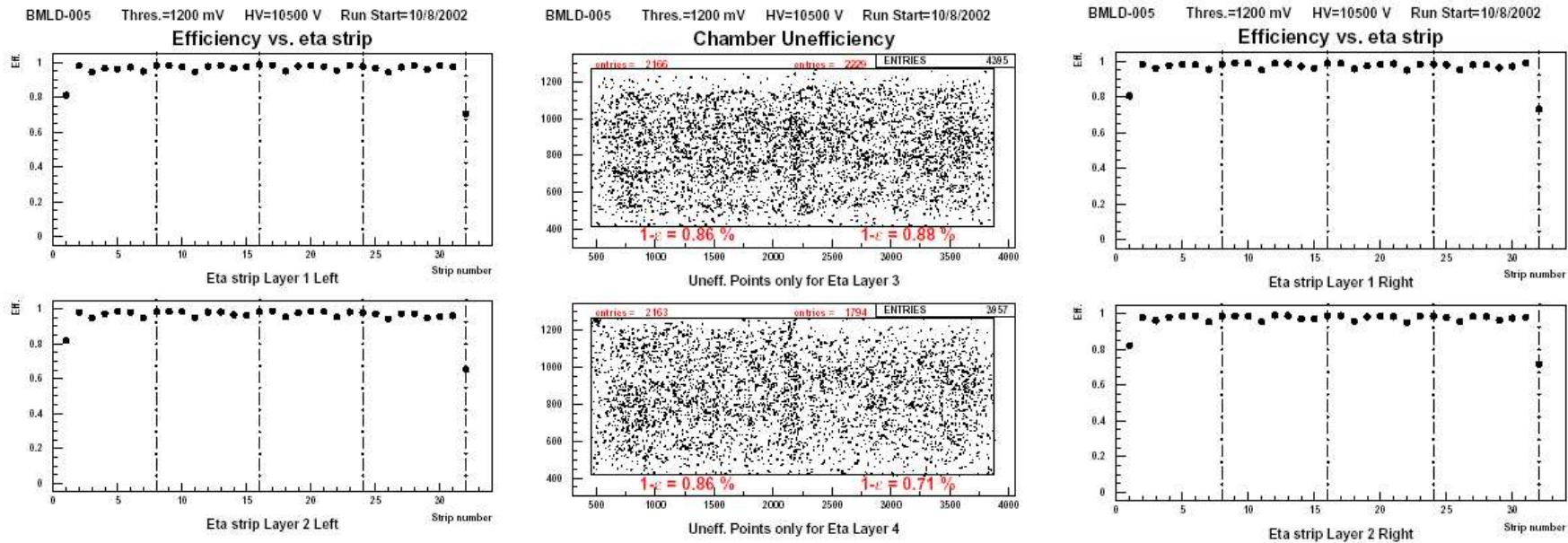
Reconstructed impact points of tracks for which **phi was measured and eta was not measured**.
