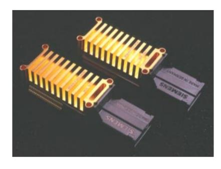
The PAROLI DC chipset is a parallel optical link developed by SIEMENS for high speed data transmission. The system consists of a TX module, a ribbon of 12 fibers and a RX module. The PAROLI TX is seen by the user as a parallel 22 bit register, clocked at a frequency which spans from 200 MHz (min) to 500 MHz (max.). It converts
