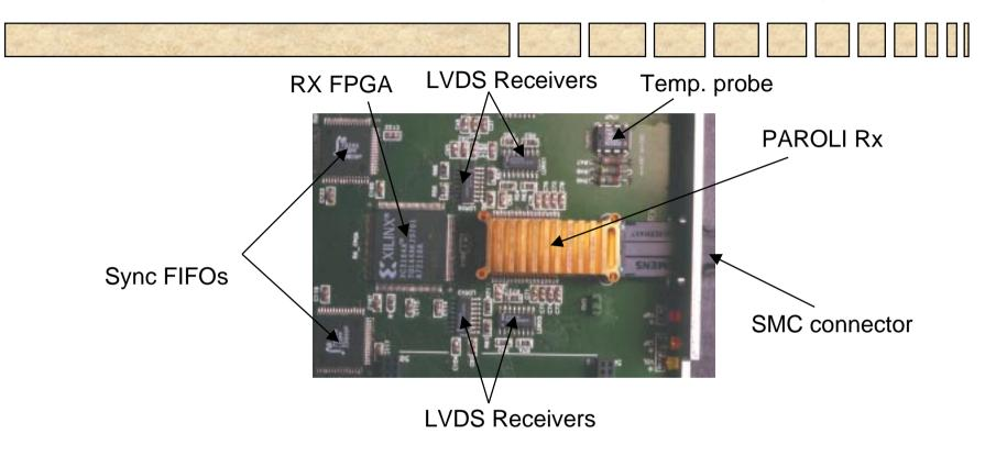
Analog issues like reflections, ground-bounce and cross-talk are also present in the RX interface. LVDS I/O standard offers low voltage swing (~ 400mV) with low power consumption and EMI.
