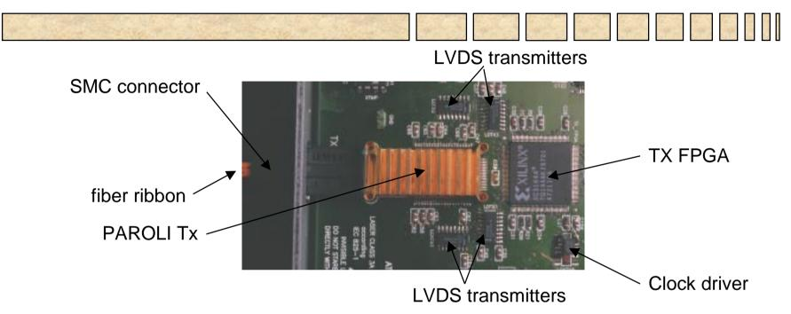
The TX FPGA performs data framing @ 200 MHz. At this clock frequency, the physical layout plays a key role in determining the digital system performance. Multi-layer boards with multiple ground and VCC planes, controlled line impedance and differential transmission scheme are required to achieve an acceptable signal integrity.
