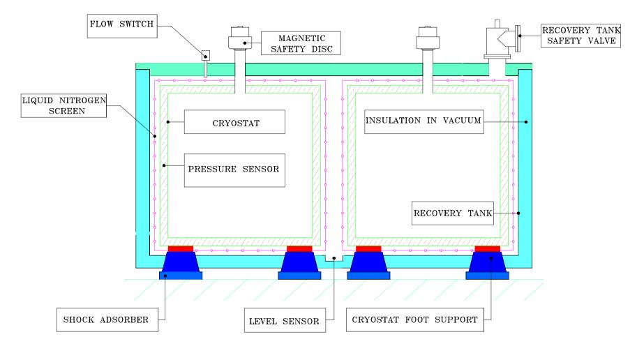
The insulation is a vacuum-tight welded box:
