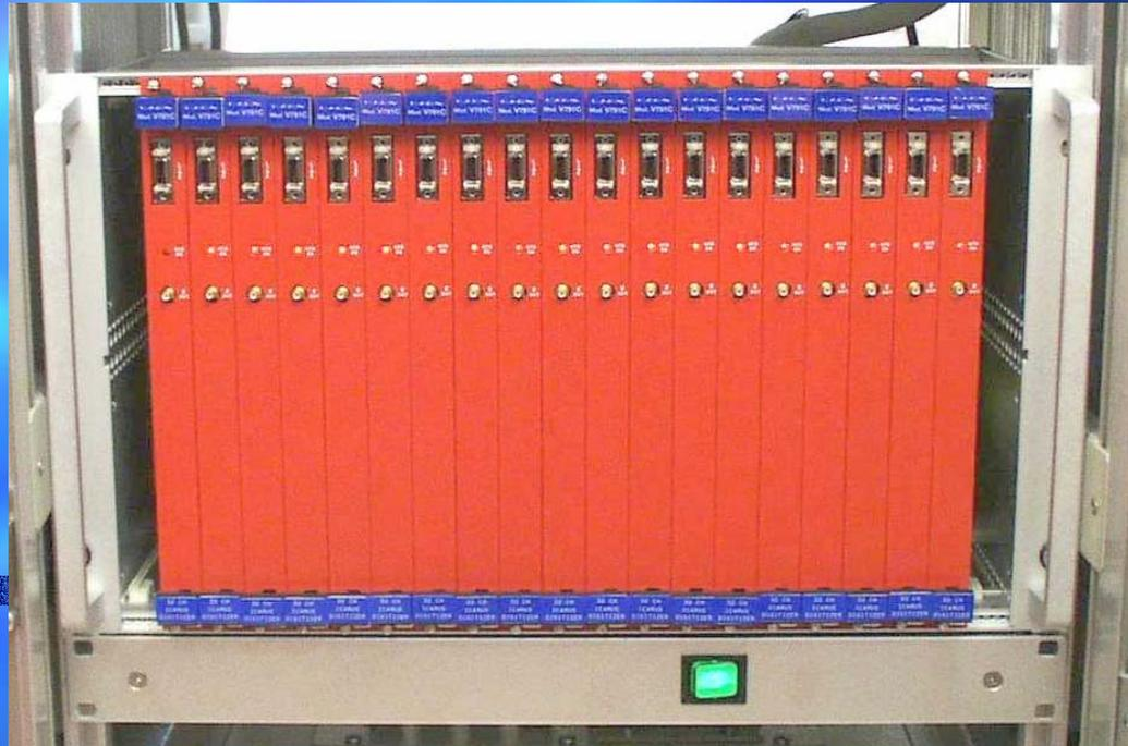
Analog crate is a standard Europa 6U-21TE. The structure has been designed in way to accommodate boards on both sides.
