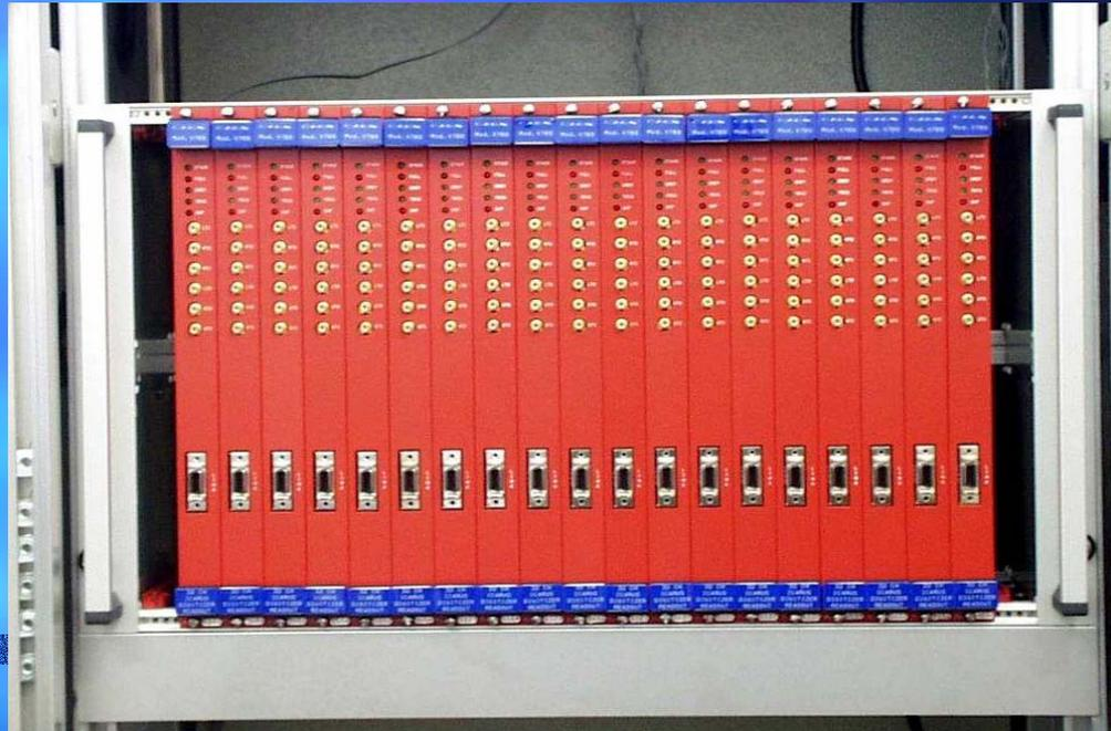
The digital crate is a standard VME crate. This crate is produced by SCHROFF and has a low EMC radiation value. Inside the crate 18 modules V789, 1 module V816 and 1 CPU are accommodated.
