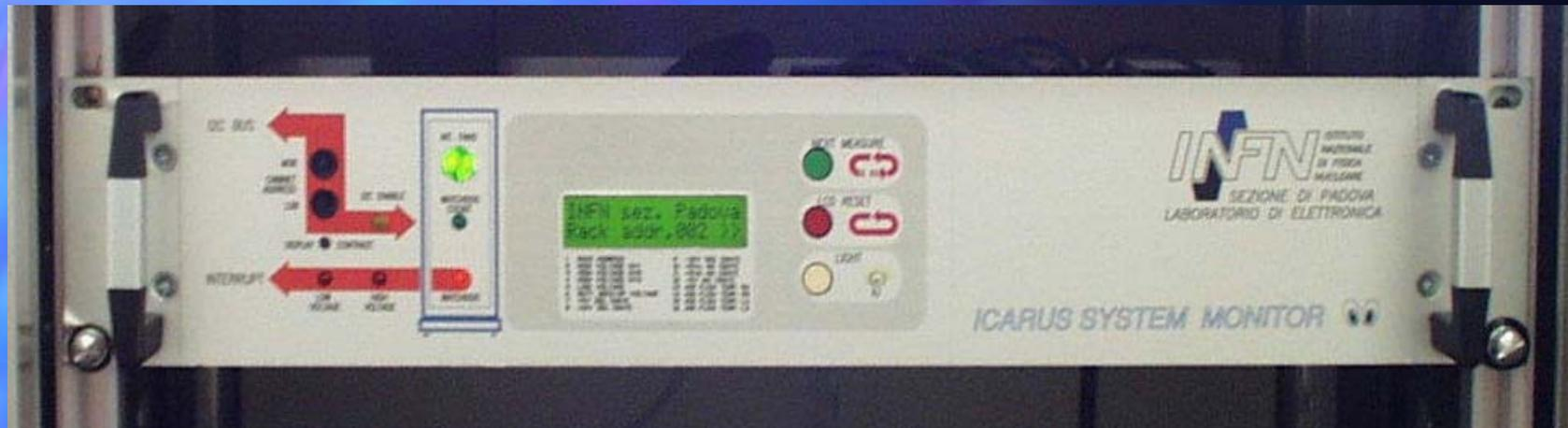
The System Monitor manages the acquisition of the rack parameters as: analog and digital crates power supplies voltages; high voltages; line voltage; internal temperatures and fans rotation.
