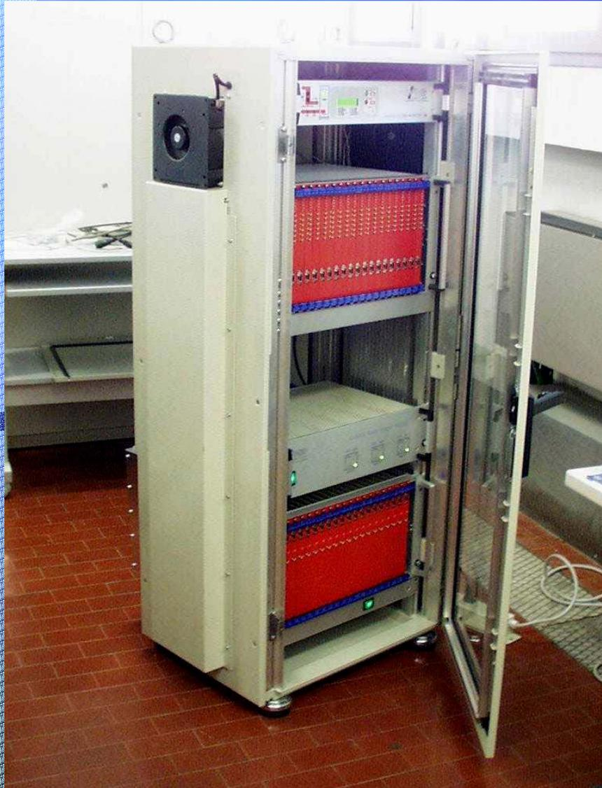
The rack has air tight structure in order to reduce post installation servicing.
