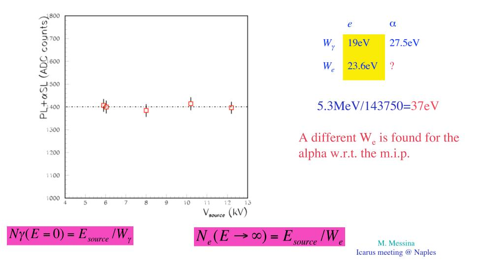
The gain factor G defined as the number of secondary photon vs. ionization electrons has been measured. It is given by the ratio of the measured SL(E->infinity) and the PL(E=0)
