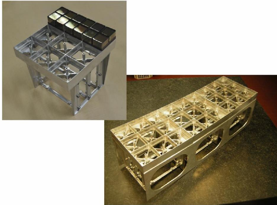
**Figure 37:** *INFN-LNF prototypes of the mechanical structure. Top Left: PDM module with 12 MAPMTs installed. Bottom Right: 3-PDM Subsection of the mechanics of the focal surface with supporting ribs. Note the sphericity of the element.*
