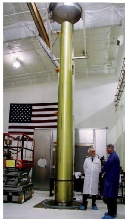
Figure 31: Expandable mast in open configuration.
