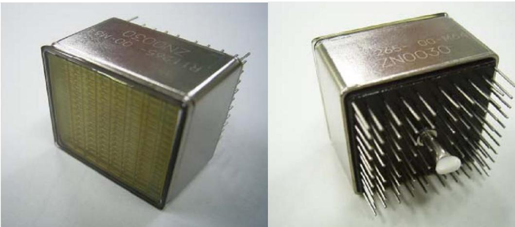
Figure 69: *Prototype of the MAPMT64*
