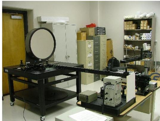
**Figure 61:** *The optical setup for the preliminary tests: the 24” parabolic mirror of the collimator is visible on the optical bench.*
