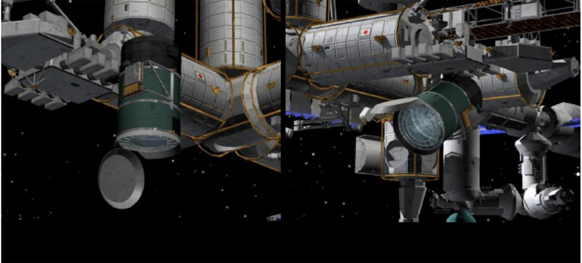
**Figure 23: *JEM-EUSO will be operated in tilted mode to increase the monitored effective area. Baseline for tilting angle is currently 38-degrees.***
